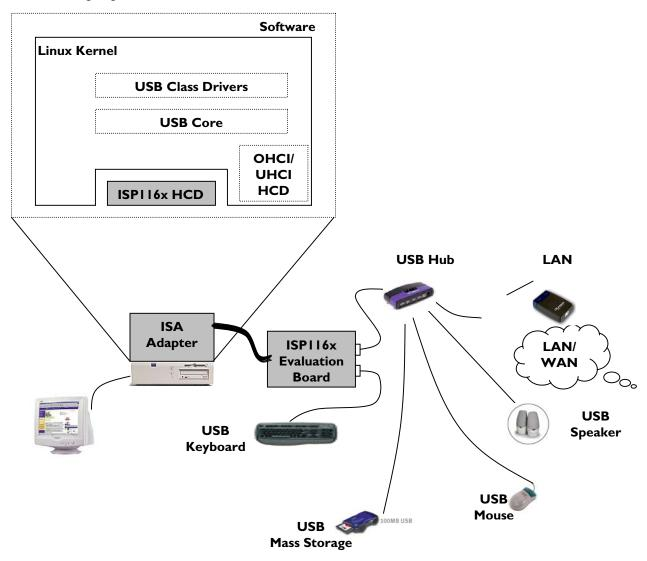
Linux kernel versions 2.4.0 and later support USB. The kernel itself provides the USB core, most of the class drivers and the USB HCDs. To work with a Linux PC, you just need to add another HCD software for the ISPI16x Host Controller. You can dynamically load or unload the ISPI16x HCD software to the Linux kernel. The interface with the USB core and the class drivers for the ISPI16x HCD is the same and this driver can work simultaneously with other USB HCDs.
